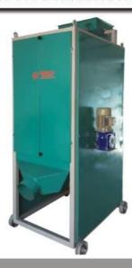
Our magnetic drum separator is very useful for removing iron impurities like nuts, bolts, heavy mild steel parts. Magnetic drum separators can be used in plastic industries, foundry, and many more industries where we can protect iron impurities from our processing plant to protect the other machineries. Drum separators are comes in ferrite & rare earth segments
